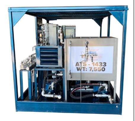
Advanced Tool & Supply's (ATS) Electric Skid Flushing and Testing Units are suitable for hydraulic pressure testing, fluid circulation, filtration, and chemical injection just as our air driven units. ATS's electric unit allows operators the option for air driven or electric when working offshore or land base. ATS's technicians are certified in NAS 1638 & 4059E and carry up-to-date certificates.
